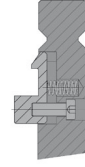
Safety-Click® Applicable for tool weight up to 12.5 kg/28 lbs. (NS I + II + AS II)
