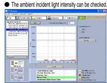
The incident light level when the light emission of the Safety Light Curtain is stopped is displayed in a bar graph.
