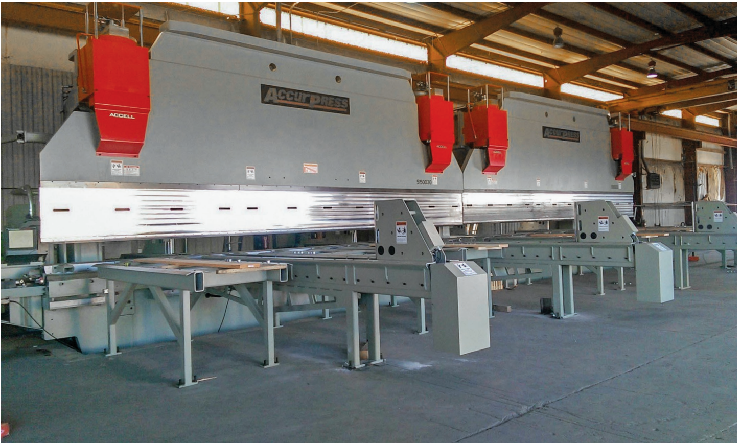
Accurpress Tandem 1500 ton by 30 ft press brakes forming 60 ft custom poles.
